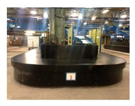
Flat Plate Carousel – each side of flat plate carousel is equivalent to one (1) pier.
